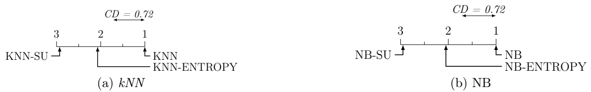
Figure 7.5: Critical differences chart for the memory consumption (RAM-Hours) obtained by weighted classifiers.
